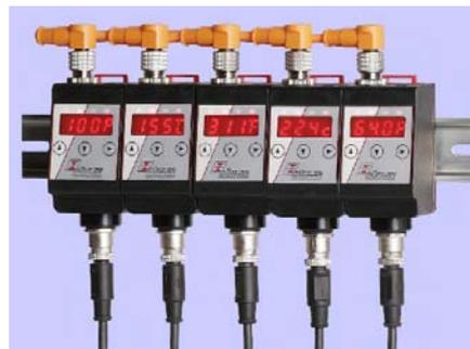
The **Multitronic** is based on the same technology and allows the remote installation of different transducers and the central installation of the controllers. Whether they display and control pressure, temperature or volume, the controllers provide the same operational mode and just need to be set to the desired standard and programmed to the required set values.
